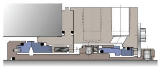
Allpac 682/QB seal for mid-range service and barrier pressure up to 51.7 bar (750 psi)
