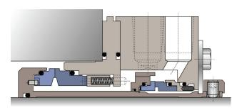
Allpac 682/ISC2-XP seal for low-duty service and barrier pressure up to 20.7 bar (300 psi)
