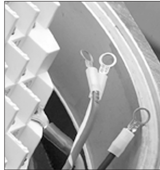
Figure 3.10: Ring tongue connectors
