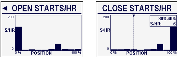
Figure 7.10: Open and close starts/hr histograms. Close starts/hr histogram displays optional bin s/hr and position values.
